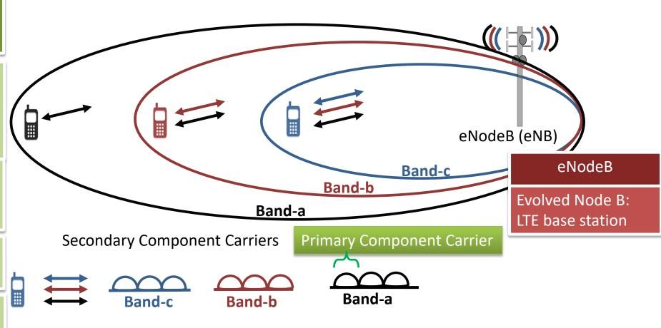
Up to 5 Carrier Components (CC) for downlink and uplink
